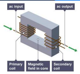
The **number of turns** on each the transformer will determine if it is a **step-up** or **step-down** transformer
